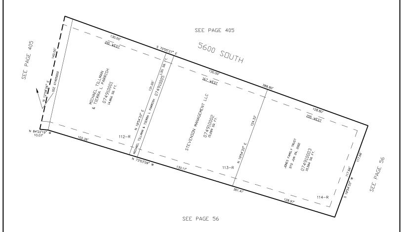
10' UTILITY & DRAINAGE EASEMENTS EACH SIDE DF PROPERTY LINES AS INDICATED BY DASHED LINES EXCEPT AS OTHERWISE SHOWN.
